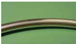
Figure 2: Parker Hannifin's Silver-Indium diffused plating
