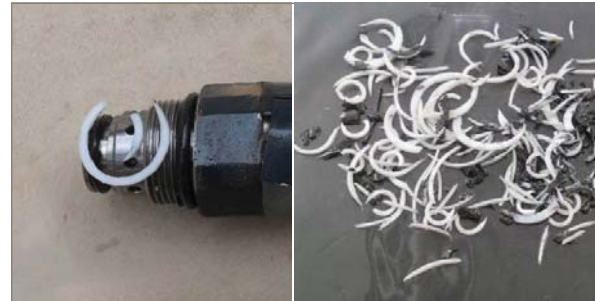
PTFE back-ups are pinched and broken during installation; leading to seal failure.
