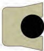
Standard PolyPak Cross-Section
