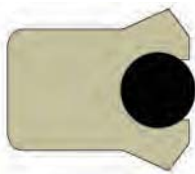
Type B PolyPak Cross-Section
