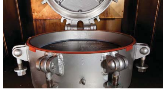
Figure 1: Alignment tabs (4) located on outside of manway nozzle.
